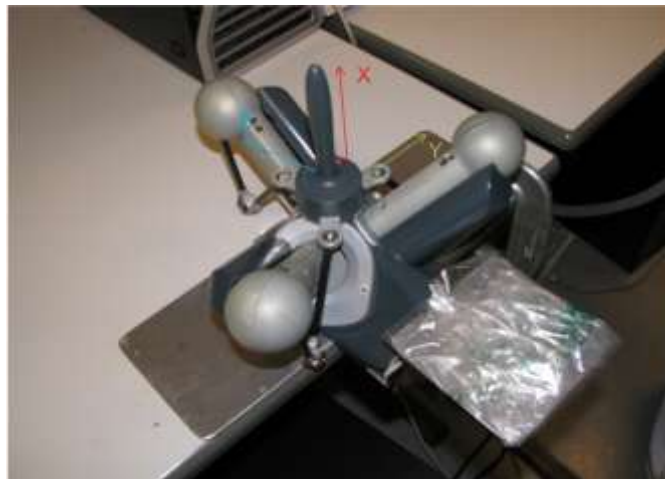
Figure 2-8. Axes directions for the referent frame of the haptic device.
